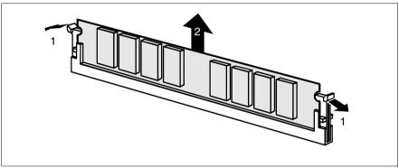
Figure 4: Removing a memory module
